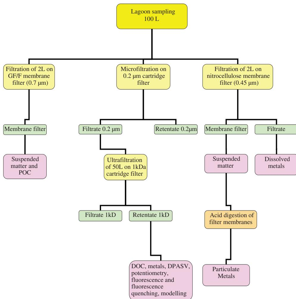
Figure 2. Schematic sampling procedure used and chemical analyses.
