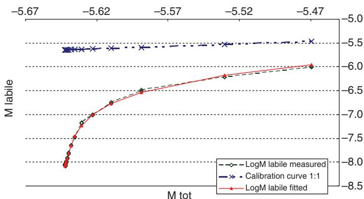
Figure 3. Experimental and fitted polarographic data for the D65 sample (25°C) (M: concentration of metal in mol L<sup>-1</sup>).
