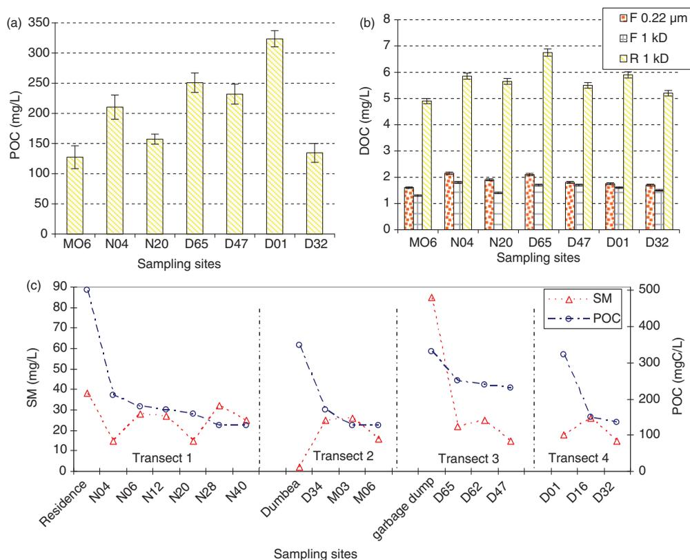
Figure 6. Evolution of (a) POC, (b) DOC and (c) SM in the various sampling sites (mg/L) (F1kD and R1kD: Filtrate and Retentate 1 kD; F0.22: Filtrate 0.22  $\mu\text{m}$ ; POC and DOC: Particulate and Dissolved Organic Matter; SM: Suspended Matter).
