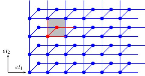
**Figure 14.** Planar structure leading to Cosserat model.
