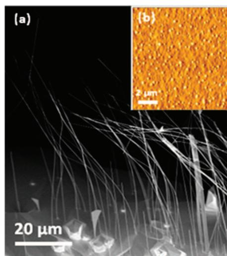
FIG. 1. (a) Top view SEM image of the (001) GaAs substrate edge showing GaAs nanowires a few tens of micrometers long, oriented along the (111)B direction, grown by Au-assisted VLS-HVPE at 715  $^\circ\text{C}$  during 30 min. The NWs were bent when exposed to the electron beam. (b) As an insert, AFM image of the surface of the Au-covered GaAs (001) substrate after annealing between room temperature and growth temperature (715  $^\circ\text{C}$ ) in the HVPE reactor.
