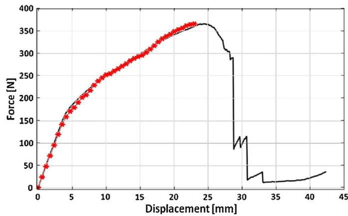
**Fig. 36** Force versus applied displacement for a uniaxial bias extension test of an aluminum pantographic sheet. The black curve is the experimental measurement and the red obtained via numerical simulation (color figure online)
