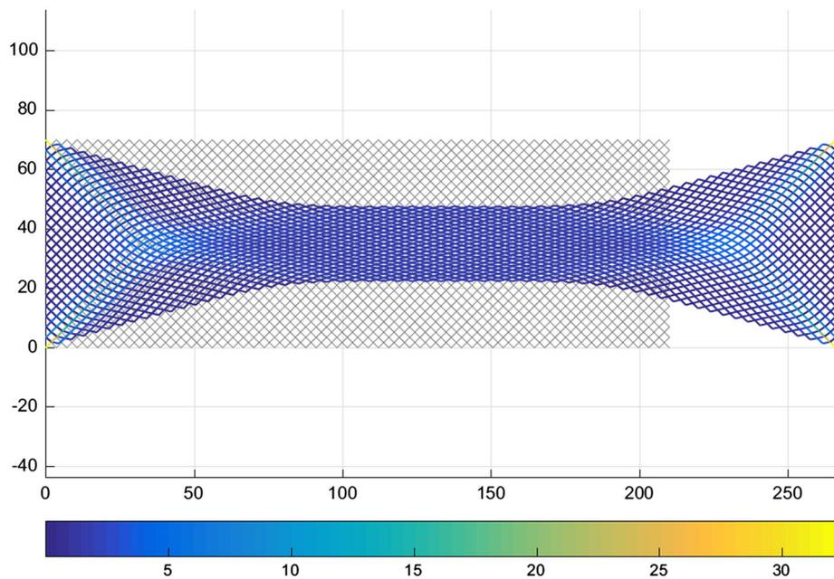
**Fig. 12** Bias extension test simulation using the micromodel when  $M = 20$  and  $N = 60$ : reference configuration (gray), current shape and color bar of the internal forces on extensional springs [43] (color figure online)
