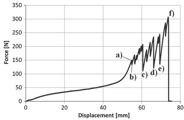
**Fig. 31** Force versus prescribed displacement for a uniaxial bias extension test. **a** Sample before first beam breakage (i.e., breakdown onset); **b** upper-left corner beam breakage; **c–f** further fiber breakage
