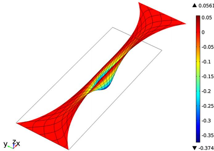
**Fig. 23** Simulation of bias extension test on parabolic pantographic fabrics. Out-of-plane buckling is observed after a critical loading. Deformed configuration and qualitative out of plane displacement
