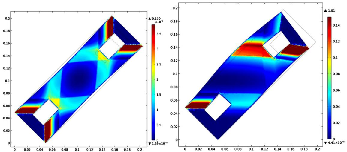
**Fig. 16** Color maps of the strain energy density for standard bias extension test (left) and combined rotation-compression test (right) of rectangular linear elastic specimen pantographic fabrics with rectangular holes (color figure online)
