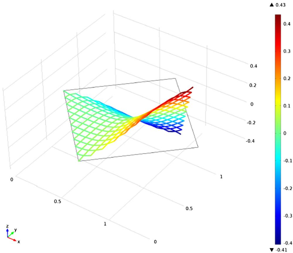
**Fig. 21** Numerical simulation of torsion of a square sheet ( $\theta = 60^\circ$ ) using the elastic surface model presented above. Colors represent qualitatively the out-of-plane component of the displacement  $u_3$  (color figure online)
