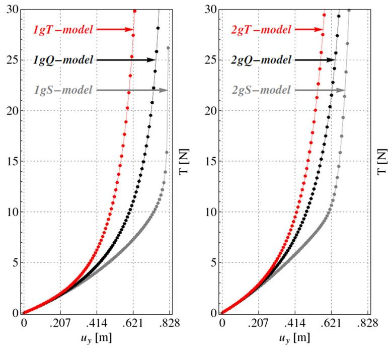
**Fig. 7** Bias extension test. Resultant (normal) forces on the short side (computed by means of Castigliano’s first theorem) versus vertical component of prescribed displacement: **a** first gradient energy models, **b** second gradient energy models
