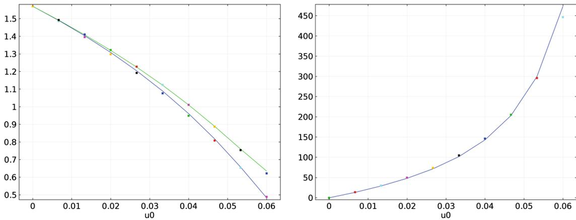
**Fig. 19** Comparisons between the Cauchy model (points) and the regression with the second gradient model (solid line). **a** Angle at the center  $\psi_C$  (blue line) and angle at the corner  $\psi_V$  (green line) on the left; **b** total reaction force (color figure online)
