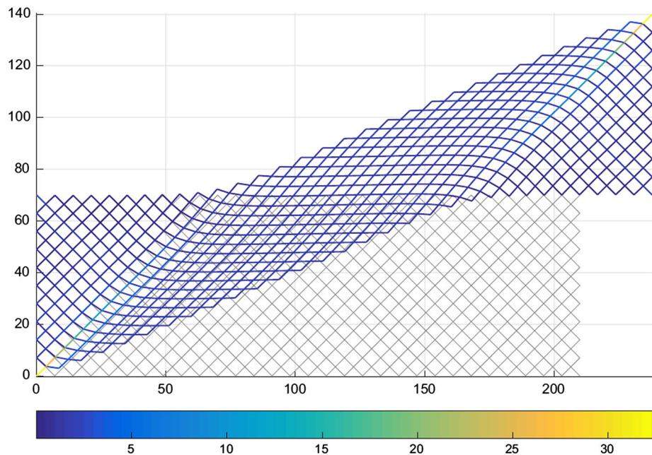
**Fig. 13** Shear-extension test simulation using the micromodel: reference configuration (gray), current shape and color bar of the internal forces on extensional springs for  $M = 10$  and  $N = 30$  [43] (color figure online)
